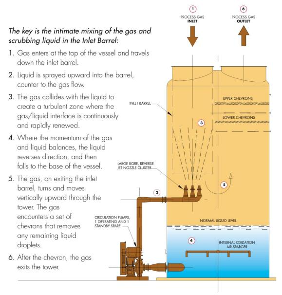
A standing wave of highly turbulent flow, called the Froth Zone, is created at the point the liquid is reversed by the gas. The Froth Zone creates a very high rate of liquid surface renewal and efficiently quenches the gas to the adiabatic saturation temperature and absorbs the SO<sub>2</sub>. Even under upset conditions, the scrubber is capable of quenching hot gases up to 1,200°C. In addition to quenching and acid gas absorption, the *DynaWave* scrubber also efficiently removes particulate.
