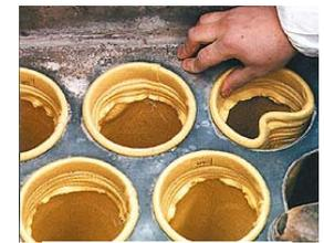
Snap-fit into the tubesheet
